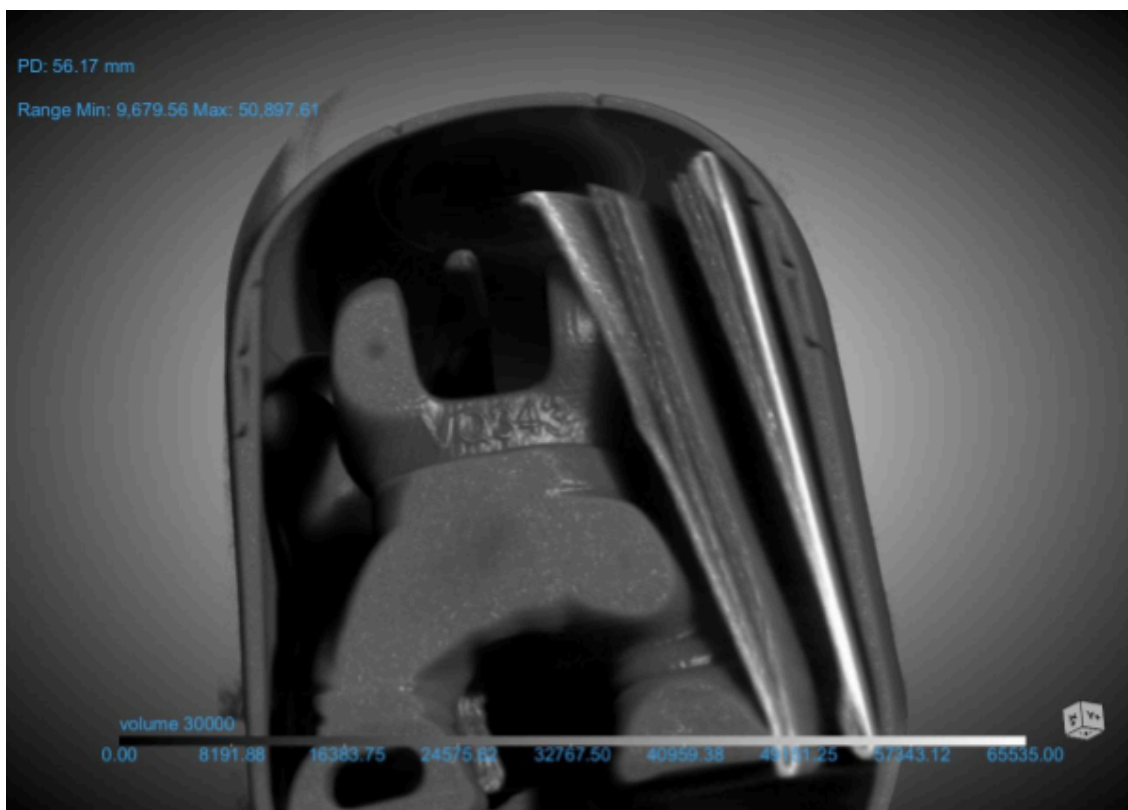
Figure 3: Processed scan of the kinderegg. Note the readable model number.
